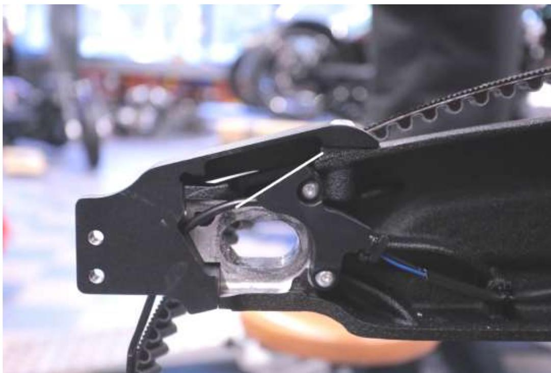
Install the new turn signals and a new tail-/brake light and connect them to the wiring. Mount a new reflector in center to the bike.
