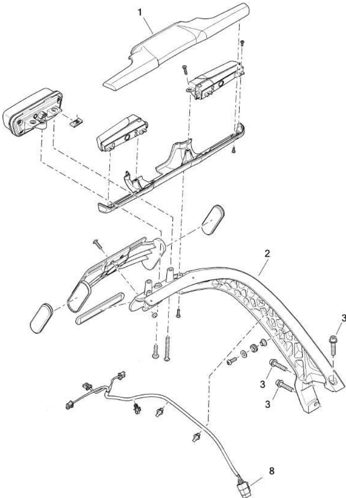
Remove the rear lights (1), the mud flap fender and the side mounted bracket (2). Remove the bolts (3) and disconnect the cable connection (8).
