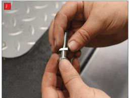
I) Remove the original fitting from the foot peg. Do not open or move the foot peg whilst this fitting is removed.
