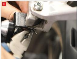
Q) Once happy with the alignment of the exhaust, start from the from of the system working your way back, tighten all fittings.
