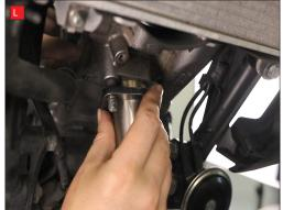
L) Loosely fit the header pipe to the bike.
