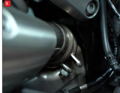
A) Start by removing the bolt from the vband clamp on the rear silencer.
