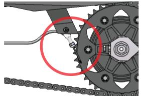
3. Secure the Dispenser Assembly to the Dispenser Plate by clamping around the black nylon sleeve using the Dispenser Plate Clip.
