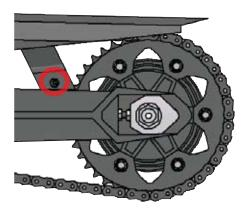
1. Remove the rear chain guard mounting bolt. Generally it is not necessary to remove the chain guard itself.
