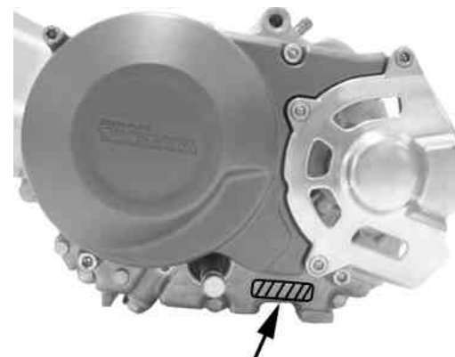
Engine No. stamped here. 4SMP-10***
