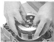
Install a thrust washer and a standard nut onto the main shaft.
