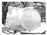
Remove the following: Oil filter rotor cover, oil filter rotor, primary drive gear, clutch lifter plate, clutch assembly, and clutch outer COMP.
