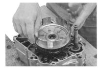
3 . Install a washer and a spline washer in this order onto the clutch outer.
