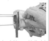
Loosely tighten an original hex bolt which holds the crankcase on the cylinder side.
