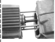
Compressing the piston rings, install the cylinder with care not to move the piston-ring end gaps out of place. Their end gaps will not be out of place.
