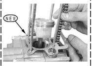
Fix a new rubber packing (black) of the kit onto the oil-return hole on the cylinder base of the crankcase.
