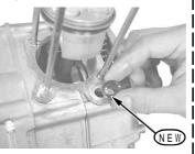
Apply engine oil to the entire inner surface of the aluminum cylinder bore.
