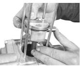
Plug the sleeve hole and the cam chain hole on the crankcase with a clean cloth, and fix a piston pin circlip.
